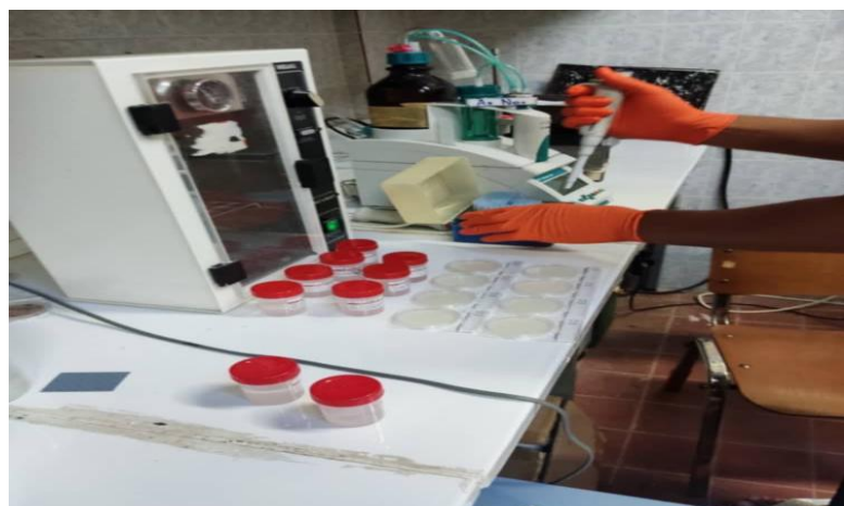
Figure-5: deposit 1 ml (1000µl) of water sample in Compact Dry plate
